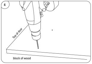
Once the handing has been chosen, remove the door using the quick release hinges. Place door on to a clean and smooth scrap piece of wood and carefully drill out the selected holes for the handle bolts.
