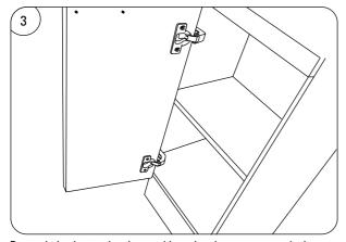
Reattach the door to the chosen side and replace cover caps in the obsolete hinge holes.  $\label{eq:cover_problem}$
