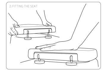
Align and insert the pins into the seat hinge sockets and firmly press down until you hear them 'click' into position. Adjustment the hinge anchors to make sure the seat line up with the edges of the toilet pan. When you are satisfied the seat is in the correct position, remove the seat from the hinge anchors (see step 3) and fully tighten the screw in the Top Fix Insert (shown in step 1) Place the Cover Plates over the Hinge Anchors. Replace the seat and click into position.
