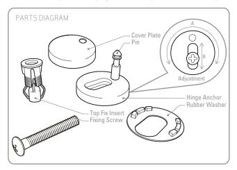
Maximum adjustment of the pin position is achieved by rotating the hinge anchor around the screw (adjustment A in the parts diagram above). Further fine adjustment of the pin position can be achieved by sliding the screw in the adjustment plate (adjustment B).
