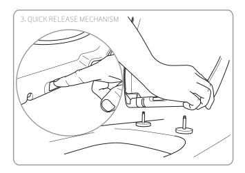
This seat is designed for quick & easy removal when cleaning the toilet pan. To activate the quick release lift the lid & seat up & press the button in the centre of the hinges & lift. To replace, align the sockets with the pins and firmly press into position.
