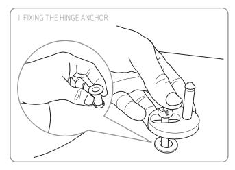
Place the Top Fix Inserts into the fixing holes in the toilet pan. Insert the screws within the Hinge Anchors as shown and begin to tighten the screws until they are loosely secured, to allow for adjustment of the seat on the pan.
