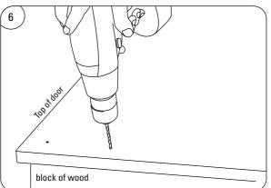
Once the handing has been chosen, remove the door using the quick release hinges. Place door on to a clean and smooth scrap piece of wood and carefully drill out the selected holes for the handle bolts. There are pilot holes to allow the handle to be fitted either vertically or horizontally.
