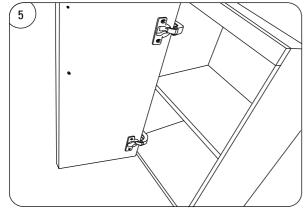
Reattach the door to the chosen side and replace cover caps in the obsolete hinge holes.
