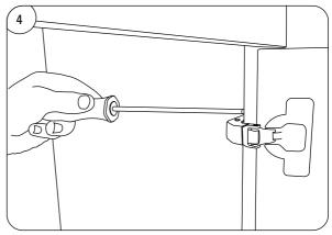
If the delivered configuration isn't suitable remove door and hinges from unit using a suitable tool.
