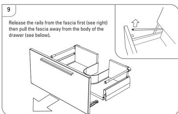
NOTE - When replacing the drawers back onto the runners ensure they have been 'clicked' back into position.
