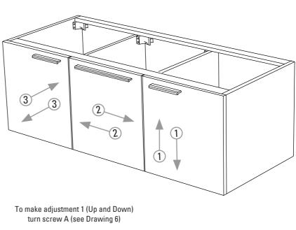
To make adjustment 2 (Left and Right) turn screw B (see Drawing 6)
