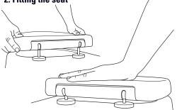
Align and insert the pins into the seat hinge sockets and firmly press down until you hear them 'click' into position.
