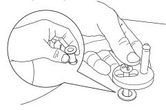
Place the Top Fix Inserts into the fixing holes in the toilet pan. Insert the screws within the Hinge Anchors as shown and begin to tighten the screws until they are loosely secured, to allow for adjustment of the seat on the pan.
