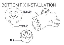
To be used with Fixing Screw, Hinge Anchor, Rubber Washer & Cover Plate if the top fix kit is unsuitable for installation.
