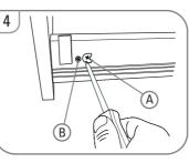
To make adjustment 1 (Up and Down) turn screw A (see drawing 4)
