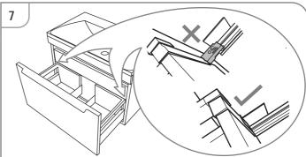
When re-fixing the drawer back to the runners, ensure that they click into position on both sides and the back of the runner is flush with the back of the drawer on both sides (see Fig.9).
