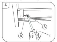
To make adjustment 1 (Up and Down) turn screw A (see drawing 4)  $\,$
