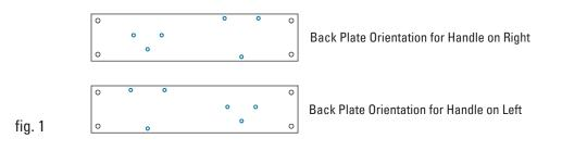
2. Once you have chosen the orientation of the handle attach the mixer valve to the back plate using the hex key fixings provided. Ensure the valve outlet is facing up. At this point install the intended initial connections (not supplied) to the valve body, so that the valve is ready to commission. Connection to the hot feed must be on the left inlet. NB - Make initial connection only, for easier connection of the final hot and cold plumbing later. (fig 2)
