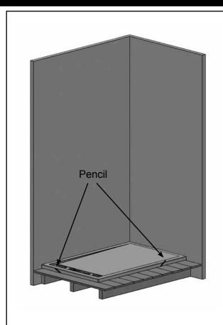
Place the tray into position, using a pencil draw the outline of the tray onto the floor boards.
