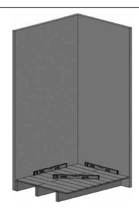
2. Ensure the floor is level (the bubble should be in the centre of the two lines on a spirit level) and free from debris.
