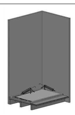
6. When the shower tray is set connect the waste pipe and check all plumbing for leaks. Once you are completely satisfied there are no leaks seal the joints between the tray and wall with a good quality bath room sealant and allow to set.
