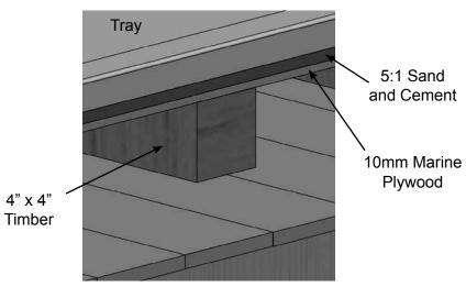
**Tip:** The exposed front where the tray has been raised up from the floor to provide adequate space for the waste pipes can be dressed using flexible plywood or plastic soffit fascia.
