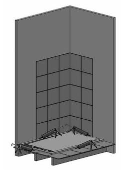
7. The tray should be tiled and grouted at this stage, seal the joints with a good quality bathroom sealant and allow to set.
