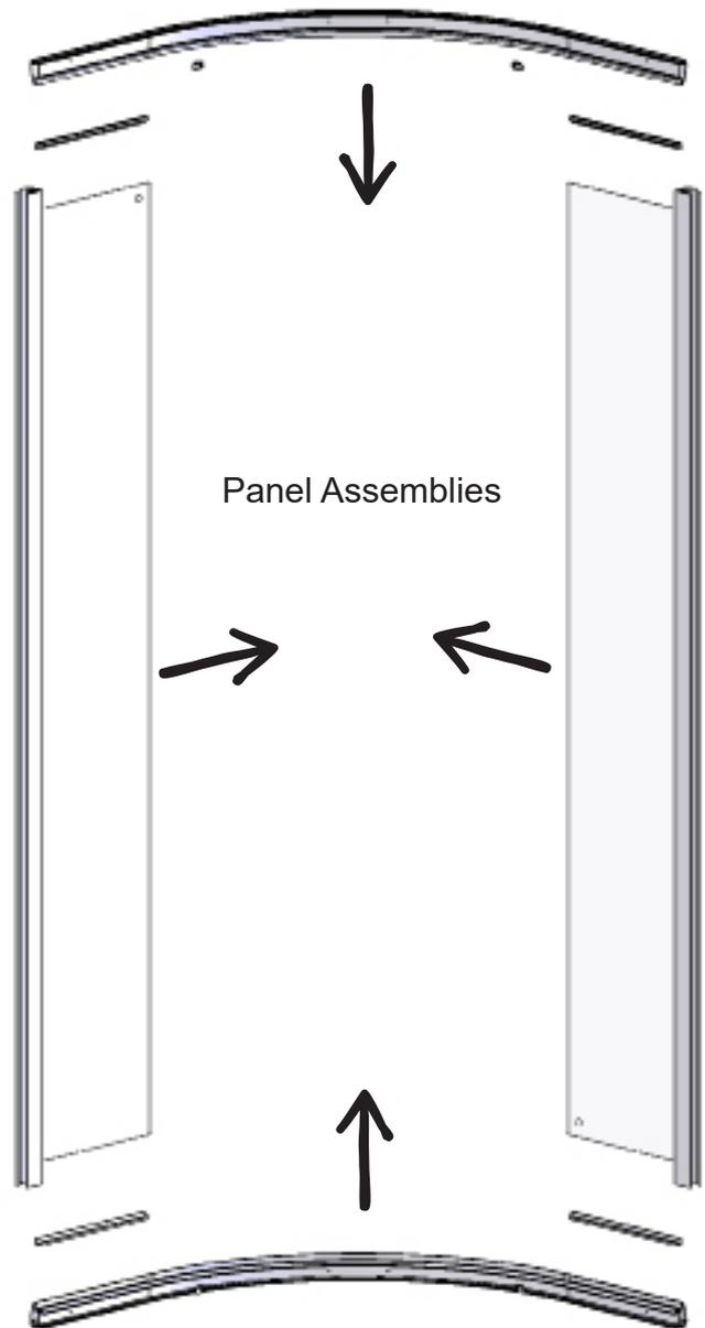
1. **IMPORTANT:** Before proceeding with this assembly remove the Red Plastic Transit blocks from the top and bottom of the Panel Assemblies and discard.
