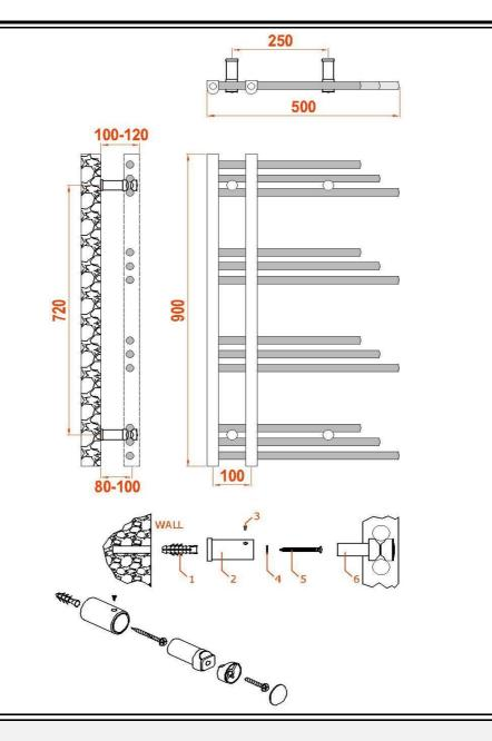
he radiator should not be mounted closer than 50mm below any overhanging surface i.ei shelf) and no lower than 100mm from the floor. Transfer the bracket drill position measurements to the
