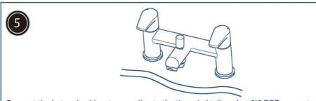
Connect the hot and cold water supplies to the threaded tails using ¾" BSP connector (not supplied). Turn on the mains water supply letting the water flow for a few minutes to flush through the system. Check all joints and connections for any leaks.
