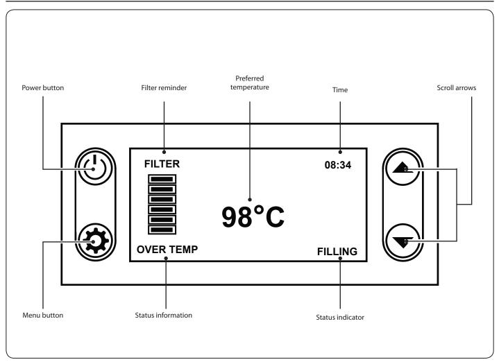
The product has a simple 4 button interface. The display will indicate the status of the boiler and the estimated remaining filter life so you know when to replace the filter. The display has a clear film cover which must be removed.
