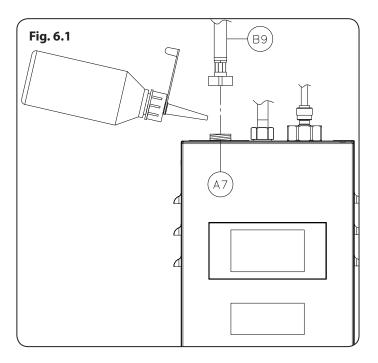
The filter system provided with this product will help to prevent of the calcification (scaling) of the boiler. However it will be required from time to time that the boiler will need to be descaled, drained and refilled to ensure the maximum energy efficiency and service life from the product especially in hard water areas. Descaling solutions can be obtained by contacting the service agent shown on the label on top of the boiler.
