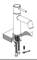
Step 2: Get out the indice behind the handle, and use allen key to remove the screw inside the handle, then take off the handle.
