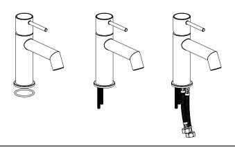
Step 7: Fix the horseshoe fixing and make sure the tap is fixed on the basin. Turn on the water supply to check if there is any leakage.
