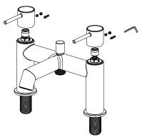
Step 5: The holes on the bathtub should be at a central distance of 180mm, the diametre of the hole should not exceed 30mm.
