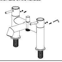
Step 3: Put the insert plates into the top of the handles, and use screw driver to fix the screws underneath the handles. PLEASE DON'T OVERTIGHEN. PLEASE NOTE THAT THE INSERT PLATE IS MADE WITH GLASS SO TAKE CARE OF IT TO AVOID IT BEING BROKEN.
