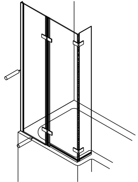
**6. FIT THE MAGNETIC SEAL BY SPLITTING THE SEAL AND ATTACHING TO THE VERTICAL SIDES OF THE FIXED AND HINGED PANEL THIS CAN BE DONE WITH THE DOOR IN THE OPEN POSITION. FIT THE BOTTOM SEAL AND BUTT THIS UP AGAINST MAGNETIC SEAL. USING A SANITARY GRADE SILICONE SEALANT SEAL DOWN THE WALL POST AND AROUND THE INSIDE AND OUTSIDE AT THE BOTTOM OF THE FIXED PANEL. LEAVE TO SET FOR 24 HOURS BEFORE USING THE BATH SCREEN.**
