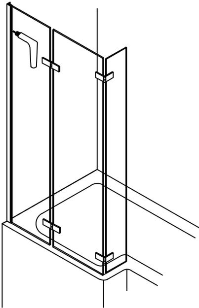
**5. WITH THE HELP OF ANOTHER PERSON PLACE THE ASSEMBLED SCREEN INTO POSITION. MARK THE POSITIONS FOR THE 3 SIDE FIXINGS (SLIGHTLY OFFSET FROM THE WALL FIXINGS SO YOU CAN FIX THE COVER CAPS) ENSURE YOU DRILL THROUGH INTO THE FIRST PART OF THE HOLLOW BOX SECTION OF THE ALUMINIUM PROFILE ON THE FIXED SCREEN BEING CAREFUL NOT TO GO THROUGH THE OTHER SIDE (DO NOT DRILL INTO THE GLASS SECTION). DRILL THROUGH USING A 3.2 mm BIT AND FIX USING THE 10mm SELF TAPPING SCREWS.**
