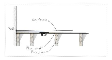
Installation using a 90mm substrate element (to be purchased separately)
