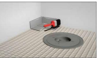
Place the waterproofing internal corners into the internal corners of the shower area and push firmly into the sealing tape adhesive. Apply a further thin layer of sealing tape adhesive over the edges of the waterproofing internal corners.
