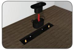
Step 16 Ease the shower drain internal bowl into the shower drain base. Ease the shower drain internal dome into the shower drain base.
