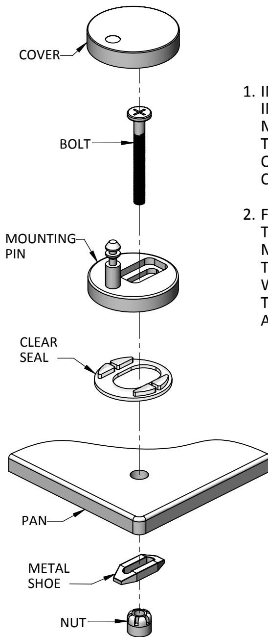
1. INSERT THE CLEAR SEAL IN THE BOTTOM OF THE MOUNTING PIN ENSURING THE SLOT IS NOT OBSTRUCTED BY THE CLEAR SEAL.
