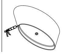
Attach waste fittings and fix your bath using white/clear bath sealant which must be applied to the bottom face of the bath. Clean off excess and be careful not to over-silicone.
