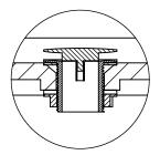
Bath A, B & C use an un-slotted waste. Bath D uses a slotted waste.
