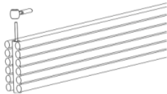
Using a hammer & steel rod to remove the centre block piece
