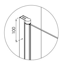
From the inside of the bath screen make a pencil mark on the wall profile approximately 100mm from the top and the bottom.
