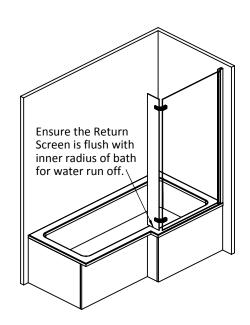
Slide the wall profile (3) onto the screen. Sit the screen onto the bath and adjust so the Return Screen butts upto the inside radius of the bath. Mark the position of the wall profile (3) with a pencil.
