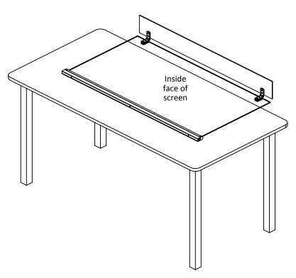
Lay front screen (1) on a flat surface to fit the return screen (2). Use the hinges provided (5). The hinge fixing screws should be to the inside face of the screen. (Do not mark the aluminium profile)
