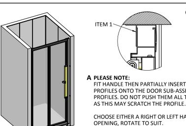
FIT HANDLE THEN PARTIALLY INSERT THE WALL PROFILES ONTO THE DOOR SUB-ASSEMBLY PROFILES. DO NOT PUSH THEM ALL THE WAY IN
