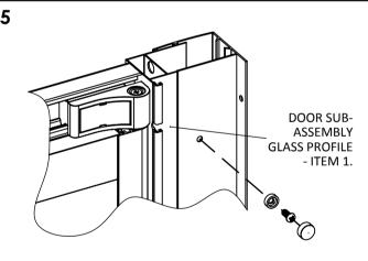
WHEN THE FRAME IS READY TO BE FIXED, DRILL THROUGH THE PRE-DRILLED HOLES IN THE DOOR SUB-ASSEMBLY GLASS PROFILES WITH A 3mm DRILL BIT.
