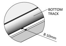
\*8-10mm IS A GUIDE FOR WHEN FITTING WITH A SIDE PANEL. FOR ALCOVE, FIT AS REQUIRED.
