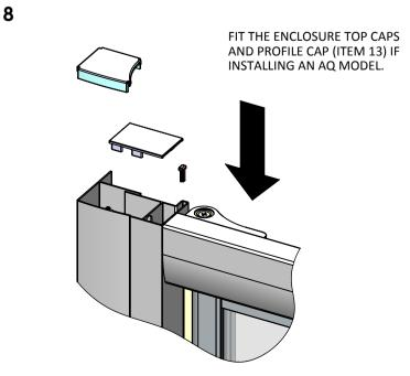
IF INSTALLING WITH AN ELLA SIDE PANEL, YOU WILL NEED TO NOTCH THE CORNER POST TOP CAP BEFORE FITTING.
