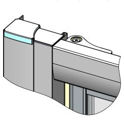
EXTERNALLY SILICONE SEAL THE WALL PROFILES WHERE THEY MEET THE WALL AND THE BOTTOM PROFILE WHERE IT MEETS THE TRAY. ALL IN A CONTINUOUS BEAD.
