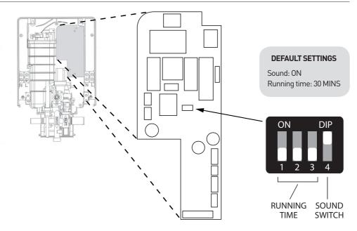
A four way DIP switch block is mounted on the main power circuit board that allows the user to configure certain shower functions. The settings can be changed on installation by moving the control PCB slider switches as described below.
