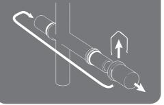
**IMPORTANT:** Before connecting the mains water supply to the shower, flush out the pipe work to remove all swarf and system debris. This is achieved by connecting a hose to the pipe work and turning on the mains water supply at the isolating stop tap long enough to clear the debris to waste.
