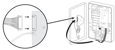
The cover can now be fitted. Please ensure that the flow control knob engages with the spindle correctly and the connector ribbon is not trapped between the covers. The front cover can now be secured with the four fixing screws provided.
