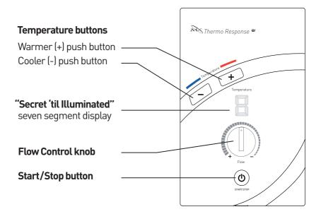
**NOTE:** the "Secret 'til Illuminated" seven segment display shines through the shower unit cover when the shower is operating to indicate the water temperature or display error codes.
