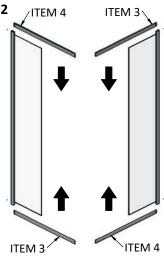
SLIDE THE TOP AND BOTTOM TRACKS; LH & RH, INTO THE GLASS PROFILES UNTIL FLUSH.
