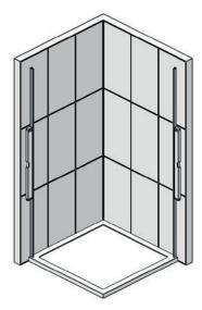
MAKE SURE THE WALL PROFILES ARE TRUE WITH A SPIRIT LEVEL. MARK THROUGH THE FIXING HOLES WITH A PENCIL. REMOVE PROFILES, DRILL AND PLUG THE WALL, (ITEM 27). THE WALL PLUGS SUPPLIED MAY NOT BE SUITABLE FOR YOUR SUBSTRATE, USE SUITABLE FIXINGS. NOW REFIT WALL PROFILES IN PLACE USING ITEM 22, 23 & 24.
