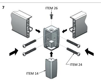
FIT THE LH & RH TRACKS ONTO THE CORNER MOULDINGS. ENSURE THAT THE TRACKS ARE SQUARE AND TRUE BEFORE SECURING THE CORNER MOULDINGS TO THE TRACK WITH ITEM 24. ALSO FIT THE CORNER MOULDING CAPS; ITEM 14, WITH ITEM 26 REPEAT FOR BOTTOM TRACK.
