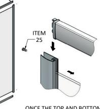
ONCE THE TOP AND BOTTOM TRACKS ARE IN PLACE USE ITEM 25 TO SECURE THE FRAME TOGETHER.
