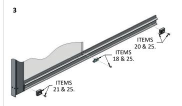
FIT THE BOTTOM GLASS CLIPS (ITEMS 18 & 19) UNDER THE GLASS. ONLY TIGHTEN SCREW PART WAY. FIT THE TOP GLASS CLIPS (ITEMS 18 & 19) AND TIGHTEN ALL SCREWS.
