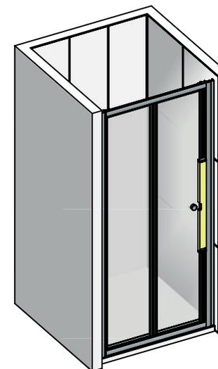
CENTRALISE THE DOOR WITHIN THE WALL PROFILES UNTIL THERE'S AN EQUAL AMOUNT OF WALL PROFILE IN THE FRAME. ENSURE THE DOOR FRAME IS TRUE AND SQUARE ON BOTH SIDES BEFORE FIXING IN PLACE.
