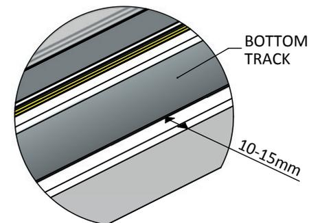
\*10-15mm IS A GUIDE FOR WHEN FITTING WITH A SIDE PANEL. FOR ALCOVE, FIT AS REQUIRED.
