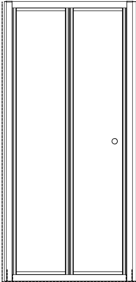
EXTERNALLY SILICONE SEAL THE WALL PROFILES WHERE THEY MEET THE WALL AND THE BOTTOM PROFILE WHERE IT MEETS THE TRAY. ALL IN A CONTINUOUS BEAD.
