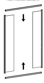
ONCE PARTIALLY ENGAGED, LIGHTLY TAP THE TRACK UNTIL FLUSH WITH THE TOP OF THE VERTICAL PROFILE.
