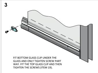
**NOTE**: THE FIXED GLASS PANELS REQUIRE A SILICONE BEAD ON THE OUTSIDE WHERE THEY ABUT THE BOTTOM TRACK.
