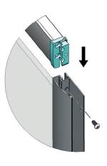
WHEN THE TRACKS ARE IN POSITION, FIT ITEM 19 THRO' THE ALUMINIUM PROFILE INTO THE TRACK END MOULDINGS (TO SUCURE THEM IN PLACE).
