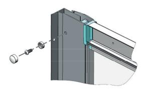
WHEN THE FRAME IS READY TO BE FIXED, DRILL THROUGH THE FRAME HOLES WITH A 3mm DRILL. (ENSURE YOU ONLY DRILL THROUGH ONE WALL THICKNESS OF THE WALL PROFILE). THEN FIX THE FRAME WITH ITEMS 19, 21 & 22
