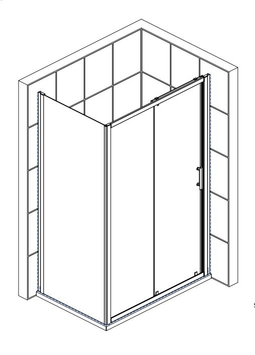
EXTERNALLY SILICONE SEAL THE WALL PROFILES WHERE THEY MEET THE WALL AND THE ALONG THE BOTTOM PROFILE AND GLASS SIDE PANEL WHERE IT MEETS THE TRAY. ALL IN A CONTINUOUS BEAD.
