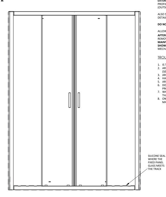
**EXTERNALLY** SILICONE SEAL THE WALL PROFILES WHERE THEY MEET THE WALL, THE BOTTOM PROFILE WHERE IT MEETS THE TRAY AND ALONG THE BOTTOM OF THE FIXED GLASS PANELS (OUTSIDE) WHERE THEY ABUT THE BOTTOM TRACK. ALL IN A CONTINUOUS BEAD.
