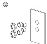
Wrapping PTFE sealing tape onto the threaded tails of the reducers and connect to the water outlet. Screw the caps over the reducers.
