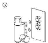
Connect the valve body with the two washers to the threaded tails on the reducers. Tighten with a adjustable wrench/spanner.
