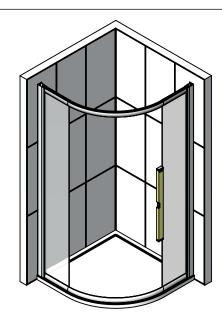
FIT THE FRAME INTO THE WALL PROFILES. ADJUSTING UNTIL THERE IS AN EVEN GAP BETWEEN THE FRONT EDGE OF THE TRAY AND BOTTOM TRACK (12mm). THERE SHOULD ALSO BE AN EQUAL AMOUNT OF FRAME IN EACH WALL PROFILE. ENSURE THE FRAME IS TRUE ON BOTH SIDES BEFORE IT IS FIXED IN PLACE.
