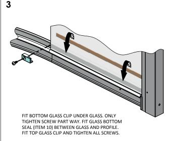
ALTERNATIVELY USE A SMALL BEAD OF CLEAR SILICONE ON THE OUTSIDE OF THE GLASS INSTEAD OF THE SEAL.
