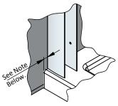
OFFER THE FRAME ONTO THE TRAY FIRST. ENSURE WALL PROFILES WILL REACH BOTH WALLS.
