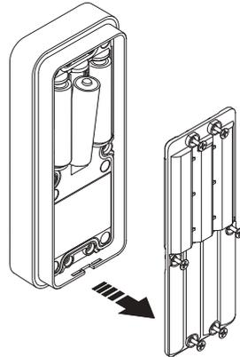
▶ When refitting the battery cover, make sure the blue seal is clean of dirt and debris. Make sure the cover is secured firmly, but do not overtighten the screws.
