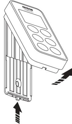
▶ Make sure the controller is dry before removing the battery cover. Turn unit over to remove the battery cover by loosening the screws with a pozi drive screwdriver.
