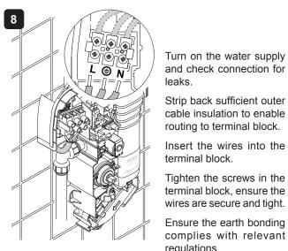
Turn on the water supply and check connection for
