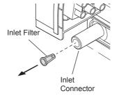
Refit the inlet filter and follow steps 7 and 10 as described in section: 'INSTALLATION'.
