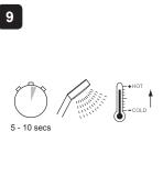
Temperature will rise further. Adjust temperature as required Note! Flow rate will reduce when temperature setting is
