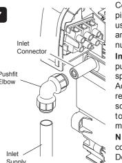
Connect the inlet supply pipe to the inlet connector using a push fit elbow or an elbow with compression nuts and olives.
