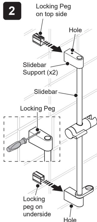
Using a suitable tool, push and hold down the locking peg through the hole in the slidebar support and pull off.
