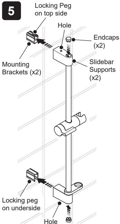
Install the new slidebar supports to the slidebar.
