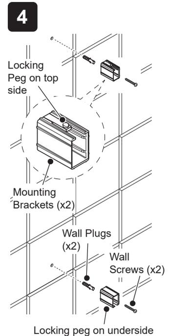
Remove and discard the existing mounting brackets, wall plugs and screws.
