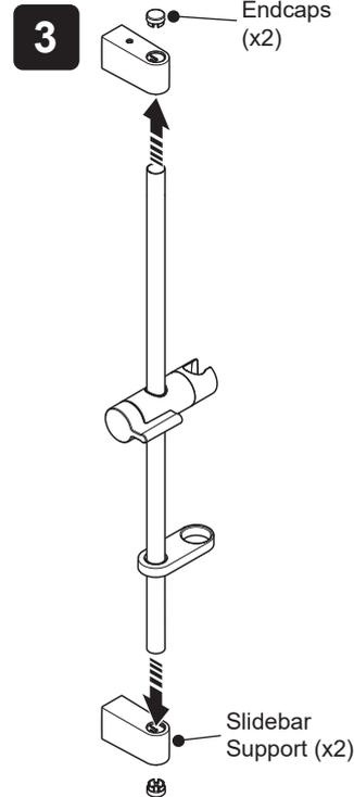
Remove the end caps and slidebar supports from both ends of the slidebar.
