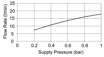
Typical Flow Rates on High Pressure Systems (with 12 Litre/Min flow regulator fitted in shower control outlet), Mira Select Flex with Mira Select Flex Shower Fittings:
