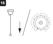
Press STOP button, light on the temperature indicator dims to standby state. When the shower has stopped running the temperature display will only show the clock. The water flow will continue for a few seconds before stopping. Isolate power. Display will go blank.
