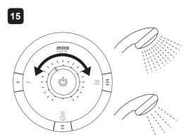
Adjust temperature as required. Flow rate will adjust automatically.
