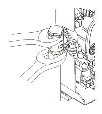
Feed cable into Case. Fit Earth sleeve (not supplied) and strip insulation.
