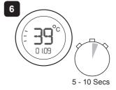
The temperature indicator becomes illuminated, showing time. Temperature will be displayed after a few seconds.
