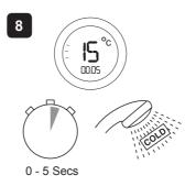
Water will be at full force and at a cool temperature as indicated by the temperature indicator.
