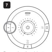
Press the 'Low' button, light on the display comes on
