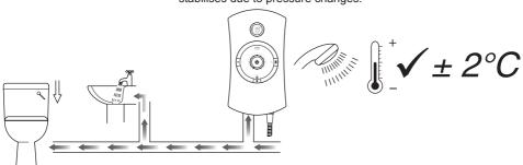
Water inlet pressure fluctuations due to other draw offs (e.g. flushing toilet). Shower temperature will be controlled to within  $\pm$  2°C of the set temperature provided that the supply conditions remain within the required operating parameters (refer to section: 'Specifications').
