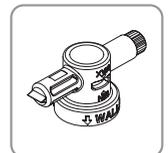
5. Remove the maximum temperature peg from the top of the valve by using a screwdriver. Refit the handle.
