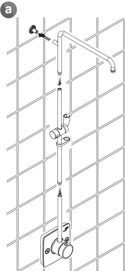
Push the clamp bracket buttons down and slide the bracket and hose retaining ring onto the middle bar, and then screw the middle and lower bar sections together. Push fit the riser arm to the middle and lower bar section.
