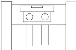
\* Pipework that is not level will make final assembly of the valve very difficult
