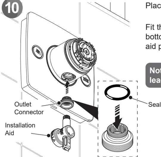
Place the seal onto the outlet connector.
