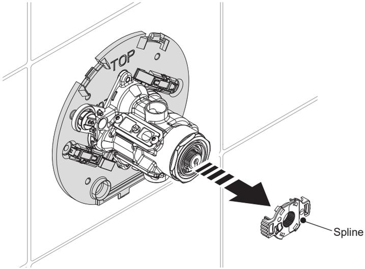
Carefully pull out the spline along with the lug from mixing valve.
