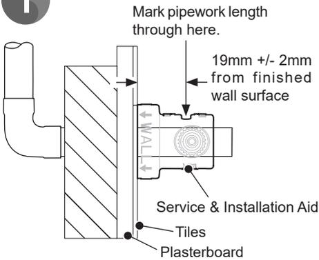
Place the service & installation aid over each pipe and using the cut out, mark the pipe for optimal length and cut pipe using a pipe Slice.
