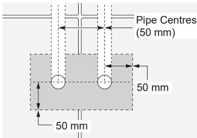
Ensure you have enough pipework through the wall to allow it to be cut to the specified length when wall is finished (A minimum of 150 mm is recommended).
