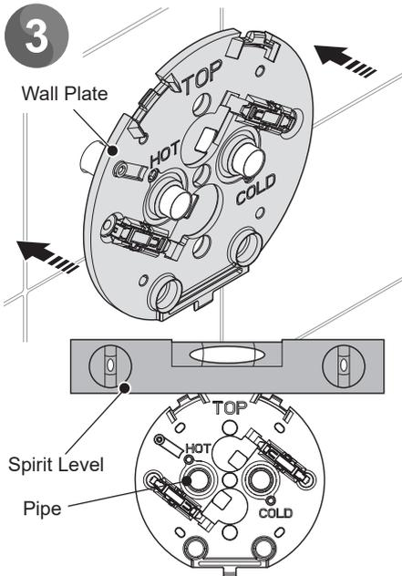
Fit the wall plate over the pipes ensuring they do not push back into the wall.
