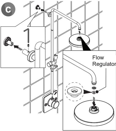
Refit the lower bar into the mixing valve and then put the concealing cover onto the riser arm mounting boss.
