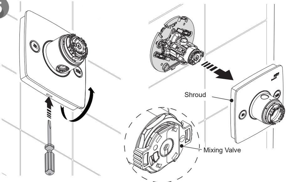
**Note:** Ensure that the mixing valve is oriented in line as shown above.
