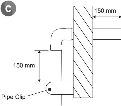
Plumb supplies using 15 mm copper pipework, make sure a minimum 150 mm of pipe extends from the front surface of the noggin (to ensure the required minimum length to fit the product).
