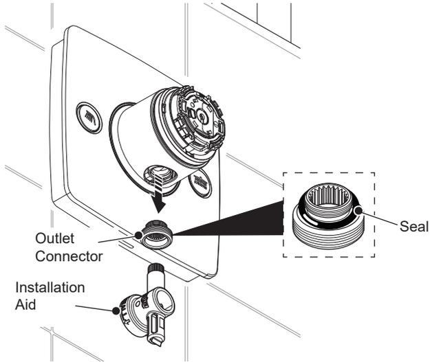
Remove the outlet connector along with the seal from bottom of the valve using the installation aid provided.
