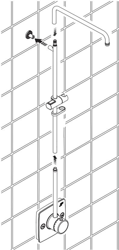
Slide the clamp bracket and hose retaining ring onto the middle bar, and then screw the middle and lower bar sections together. Push fit the riser arm to the middle and lower bar section.
