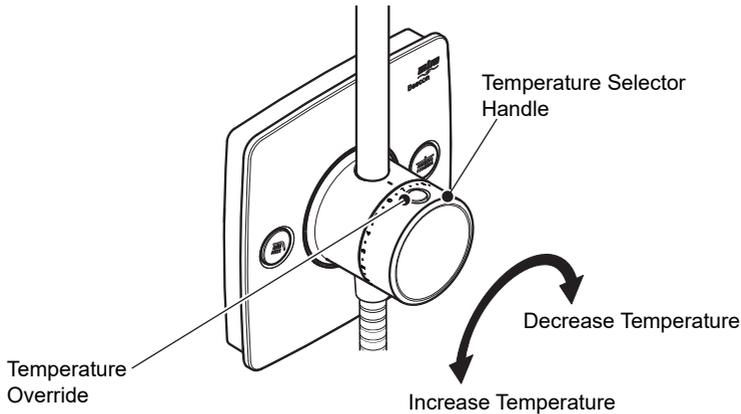
The temperature is controlled by rotating the temperature handle. Operate the shower and make sure it delivers cold water initially and then further rotate to increase temperature, for safety reasons, the temperature is limited by an override stop. To obtain a higher temperature, press the override button on the temperature handle and continue to rotate the handle. Rotate the handle anti-clockwise to turn the product off.
