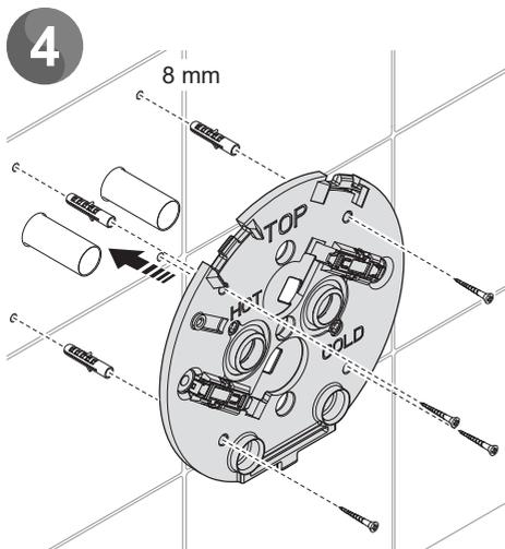
Drill the four 8mm holes and insert the wall plugs.
