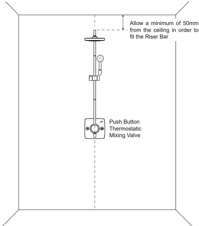
**Note:** If installing in a restricted height area a short bar can be ordered as a spare part.
