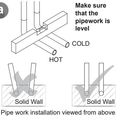
Pipework must be at 50 mm centres, level and perpendicular to the finished wall surface.
