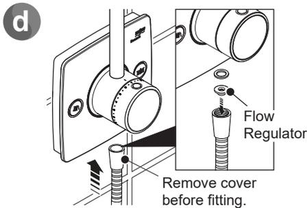
Fit the shower hose onto the bottom outlet of the mixing valve. (Install the flow regulator if required).
