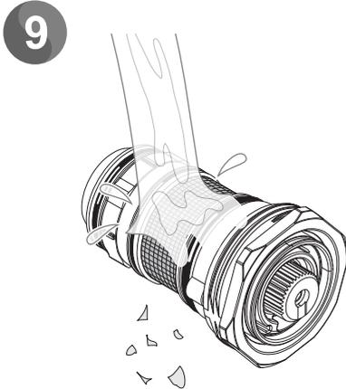
Rinse the filter in clean warm water, removing any dirt or debris.
