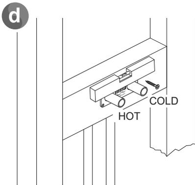
Once the pipework is in place, slide the First Fix Pipe Guide over the protruding pipework.
