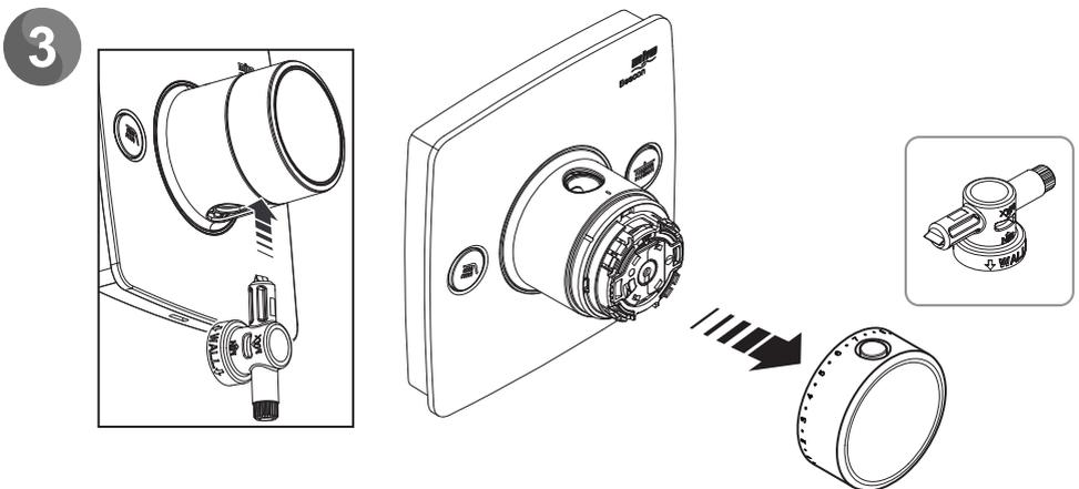
Remove the handle by using the blade on the installation aid, place in between the bottom of the handle and shroud and twist to unclip the handle.
