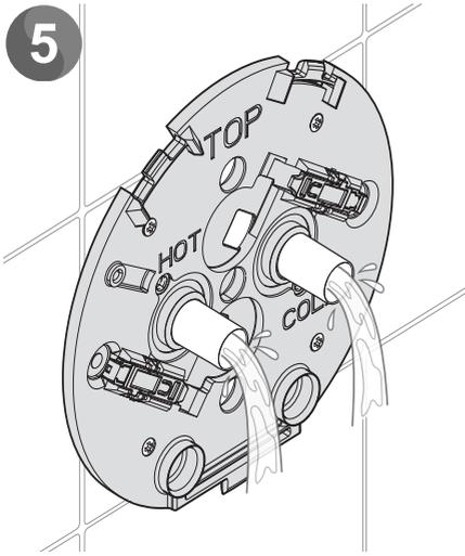
**Flush the water supplies thoroughly before connecting the valve.**
