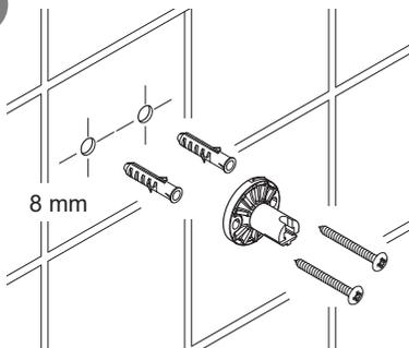
**Note: When drilling the tiles ensure this is done in the middle or towards the bottom of the marked slots.**
