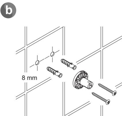
**Note: When drilling the tiles ensure this is done in the middle or towards the bottom of the marked slots.**
