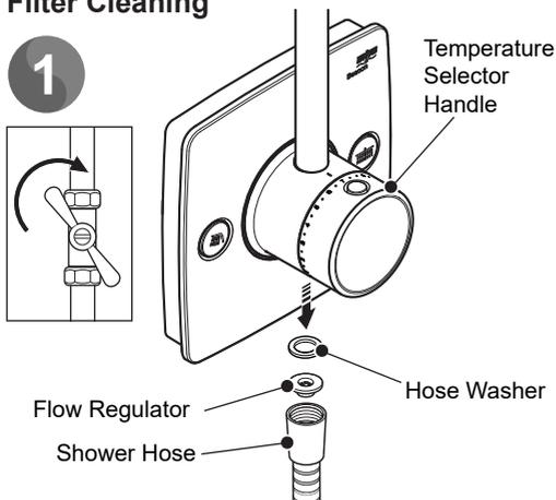
Isolate the water supplies and turn the shower on to relieve the water pressure. Turn the shower off.
