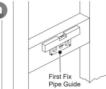
For stud partition wall installations, make sure that a wooden noggin is in place directly behind the final valve position.
