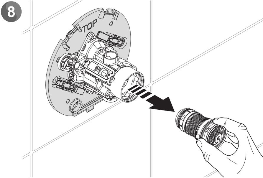
Carefully pull out the cartridge from the valve body.
