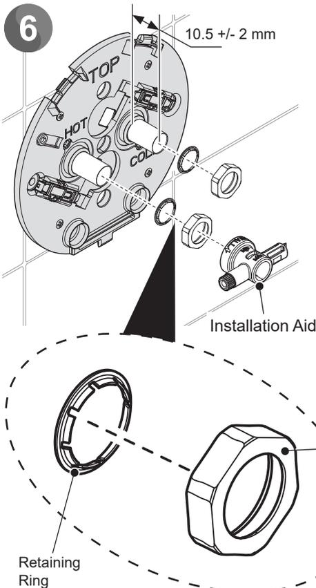
Place the retaining rings and nuts over the pipes in the orientation shown and tighten in place using the installation aid.
