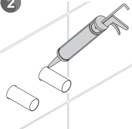
Apply silicone sealant according to the manufacturers instructions to the pipework where it comes through the wall.
