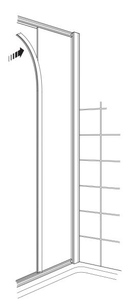
(a) Install the seal to the glass panel.
