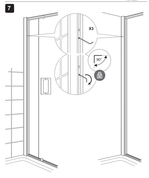
(a) Using the 3.0 mm hexagonal wrench (supplied), turn through  $90^{\circ}$  clockwise to lock the door frame, corner post and side panel in position.
