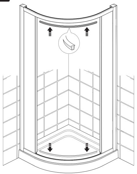
(a) Install the flexible track infill strip to the top and bottom tracks.
