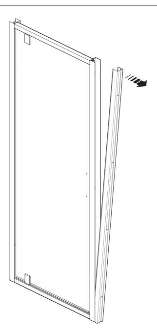
(a) Remove the wall channel.from the door.
