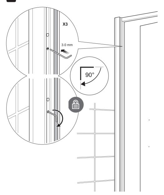
(a) Using the 3.0 mm hexagonal wrench (supplied), turn through 90° clockwise in three locations to lock the door frame in position. Repeat this on the other wall channel.
