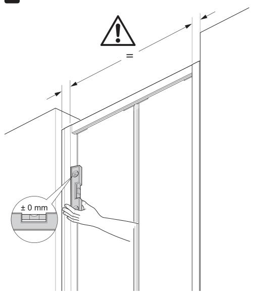
(a) Centralise the door frame within the wall channels, making sure that the door frame is square.
