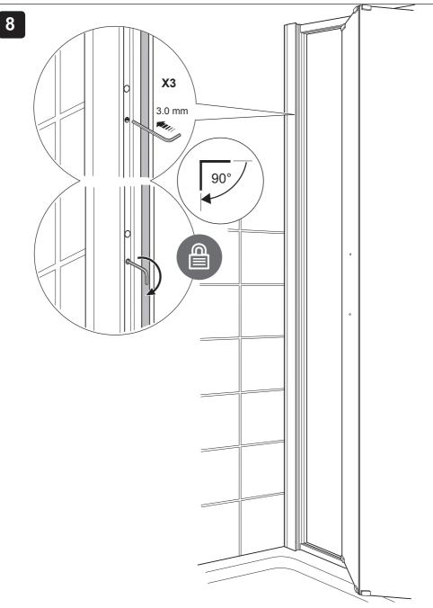
(a) Using the 3.0 mm hexagonal wrench (supplied), turn through 90° clockwise in three locations to lock the door frame in position.
