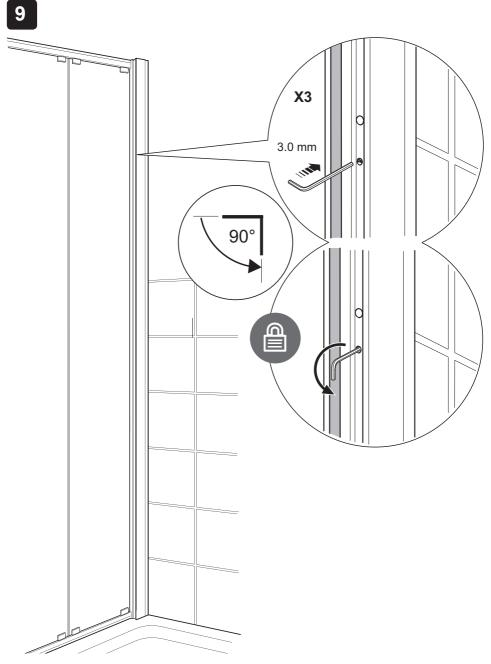
(a) Using the 3.0 mm hexagonal wrench (supplied), turn through 90° clockwise in three locations to lock the door frame in position.
