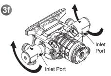
Rotate the inlet ports towards the inlet pipes.
