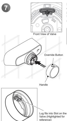
Push fit the handle ensuring that the override button is set at 12 O'clock position and the lug on the inside of the handle matches up with the slot available on the valve.
