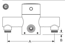
Measure the distance between the inlet face and the flat surface (Distance B) for the previously installed product.
