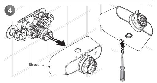
Locate the hole on the underside of a valve, and using a small flat blade screwdriver, gently rotate the screwdriver to lever off the shroud.
