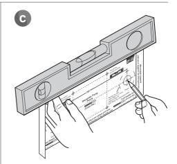
Use the template provided to mark the positions of the pipes and fixing holes.
