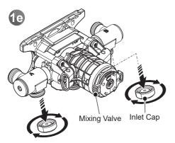
Remove the inlet caps from the optional inlet ports and retain for reinstallation.
