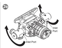
Rotate the inlet ports towards the inlet pipes.
