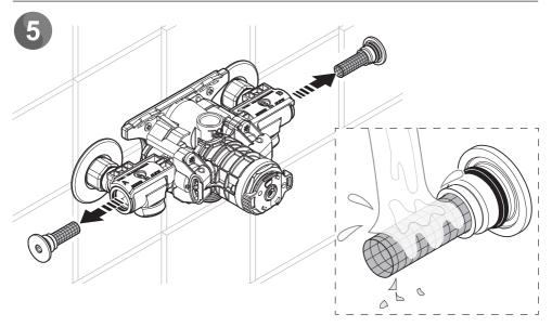
Remove the inlet filters using 6 mm hex key. Rinse the filters in clean water, removing any dirt or debris. Wipe the inside of the elbow with a clean cloth to remove any remaining debris. Replace if the filter mesh is damaged.
