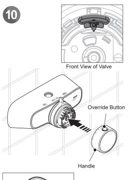
Push fit the handle ensuring that the override button is set at 12 O'clock position and the lug on the inside of the handle matches up with the slot available on the valve.
