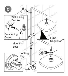
Put the concealing cover onto the wall fixing bracket.
