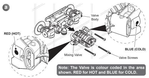
Loosen the four valve screws and remove the mixing valve from the valve body.
