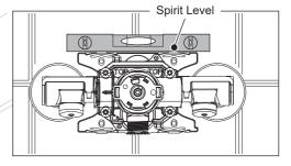
Note: Identification on the mixing valve shows the orientation that the valve must be fixed to the wall. Ensure the "TOP" marking faces to top of the product.
