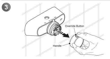
Rotate the handle clockwise until the override button faces upwards. Press the override button, and carefully pull the top of the handle away from the shroud.
