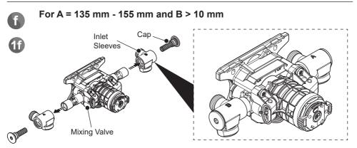
Remove the inlet sleeves using 6 mm hex key. Note the **"A"** and **"B"** markings on the inlet sleeves. Swap the sleeves and fit onto the mixing valve oriented as shown.
