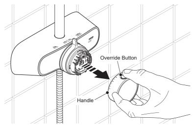
**5.** Lever out the yellow maximum temperature peg from the front of the valve by using a screwdriver. Refit the handle.
