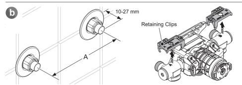
Inlet pipes must extend 10-27 mm from the finished wall surface, and be square to the wall. If pipes are longer than 27 mm cut and deburr pipe to a suitable length.
