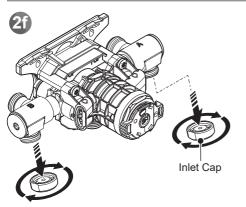
Remove the inlet caps from the optional inlet ports and retain for reinstallation.
