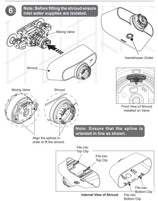
Slide the shroud over the valve and push until clipped. Ensure that outlets are in the correct position and drive features match. The shroud should click and clip into place.
