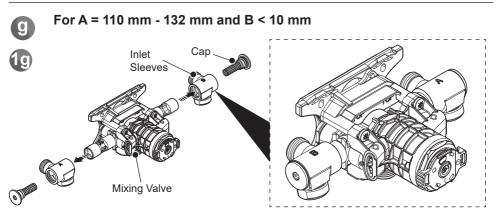
Remove the inlet sleeves using 6 mm hex key. Note the **"A"** and **"B"** markings on the inlet sleeves. Swap the sleeves and fit onto the mixing valve oriented as shown.
