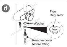
Fit the shower hose onto the bottom outlet of the mixing valve. (Install the flow regulator if required).
