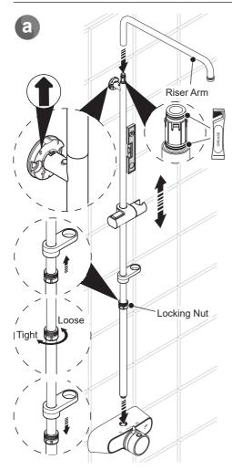
Insert the wall fixing bracket into the upper bar mounting boss, then swivel the bar if necessary to reposition the wall fixing bracket against the wall.
