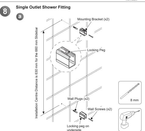
Mark the wall fixing positions and drill two holes to suit the wall fixings.
