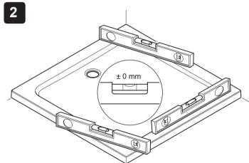
Place the shower tray on a flat surface and using a spirit level check that it is straight and flat and that the shower cubicle will sit on its surface correctly when fitted.
