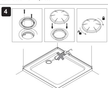
Install the waste. Tighten to ensure a correct seal. Do not overtighten. Install connecting pipework in accordance with Building Regulations. **Do not** Use silicone sealant.
