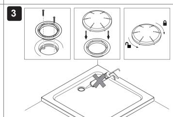
Install the waste. Tighten to ensure a correct seal. Do not overtighten. Install the connecting pipework in accordance with Building Regulations. **Do Not** Use silicone sealant.
