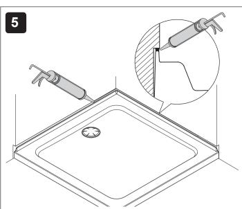
Apply silicone sealant in accordance with the manufacturer's instructions to seal the shower tray to the wall.
