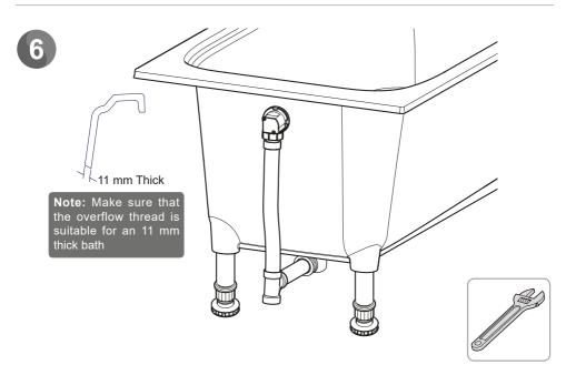
Install the drain and overflow fittings according to the installation instructions packed with the drain.
