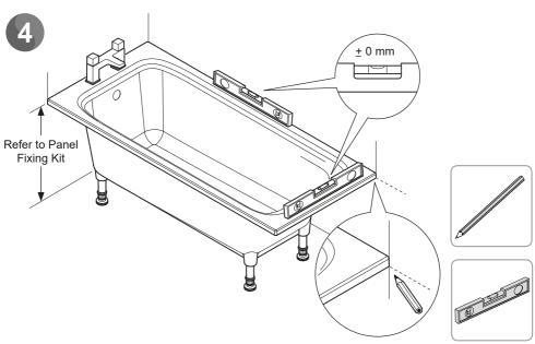
Position the bath and adjust the feet to level. Mark the position of the product.
