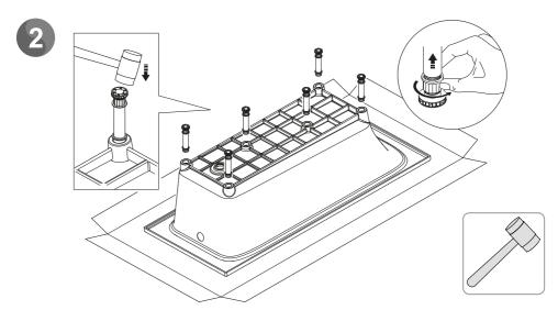
Install the adjustable feet on the underside of the bath.
