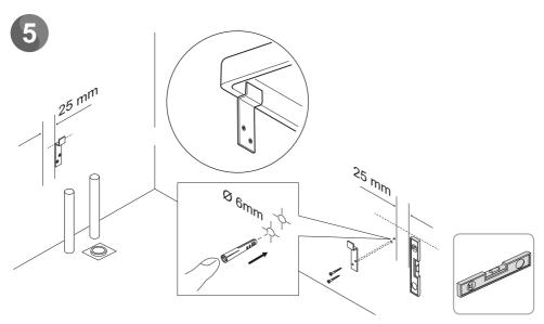
Mark and drill the fixing holes for the brackets. Install the brackets using the supplied wall plugs and screws.
