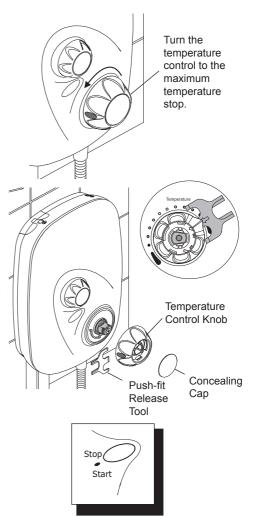
2.5. Remove the small label covering the retaining screw on the temperature hub. Unscrew the retaining screw and remove the temperature hub.
