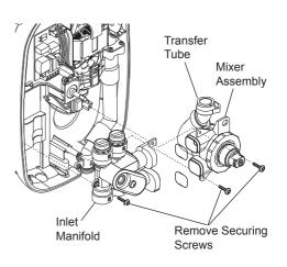
**5.9.** Inspect inlet manifold/valve interface seals and renew if required.
