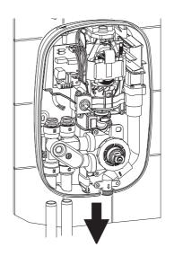
**Important!** This Mira Event XS **must** be fixed to the wall at all three fixing positions. The fixing holes are elongated to assist in vertical and horizontal alignment.
