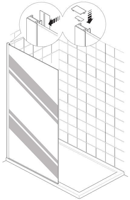
(a) Install the wall channel cover and the plastic covers.
