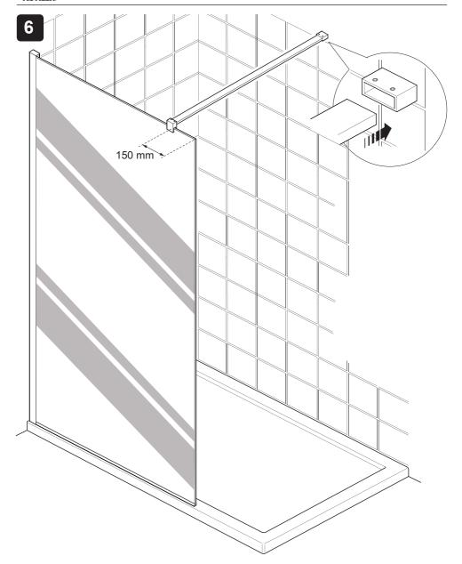
(a) Insert the bracing bar into the wall bracket.Note! The bracing bar may need cutting to length depending on the size of the shower tray
