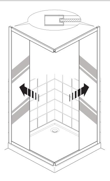
(a) Install the panel assemblies into the wall channels.
