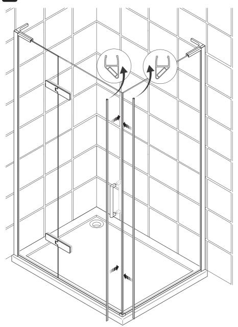
(a) Push the vertical closing seals onto the side panel and door.
