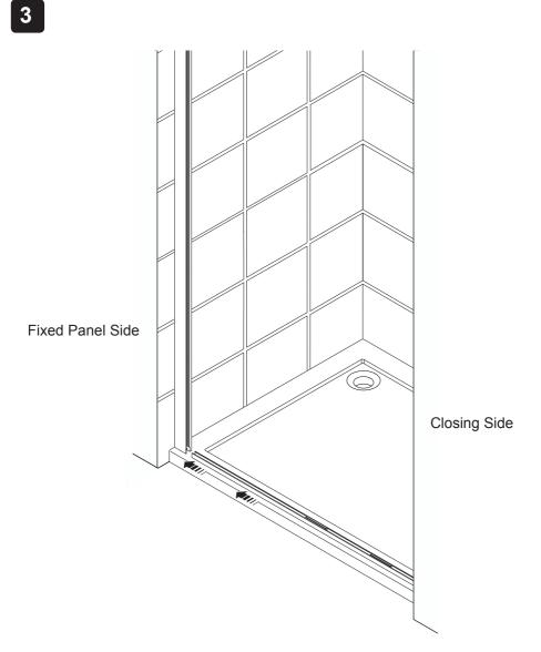
**Note!** Position the track so that the black gasket is on the fixed panel side for the glass to rest on and that the locating blocks are on the open door side.
