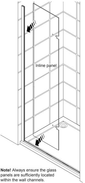
**Note!** Insert the glass noting the correct orientation. This is indicated by the label on the glass.
