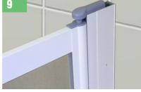
Offer the door(s) back into their respective compensators, re-align with the mark(s) you had previously made for the door position. **ENSURE** the compensator is fixed securely to the wall. Use the supplied hinge locater, FIG 7 & 8, if necessary for added rigidity.
