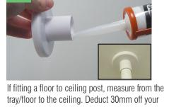
measurement and cut the post to this size. Apply a small amount of silicone sealant to the inside of the ceiling rose collar prior to fitting in place to reduce the amount of play once the post is secured. Ceiling rose has a push on cover to hide the screws.
