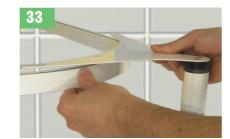
Place boomerang bracket in the top of the post, pilot drill holes in the rails top channel and fix to the post through the brackets pre-drilled holes.
