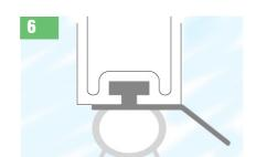
Ensure that the rubber seal on the bottom of the door(s) is slightly compressed against the tray surface or floor.
